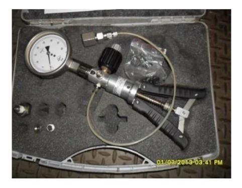
The test equipment should be calibrated ashore once a year.
