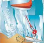
As the ship sinks, the liferaft painterline will be stretched and the liferaft starts to inflate.
