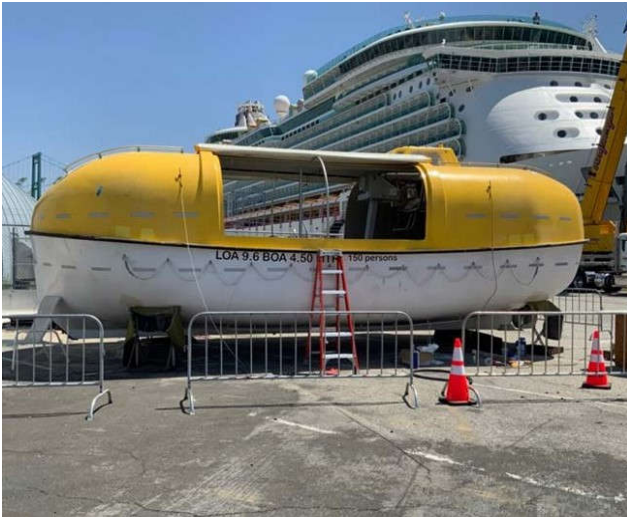
A partially enclosed lifeboat
