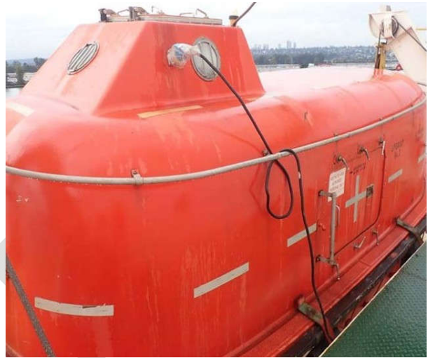
A fully-enclosed lifeboat
