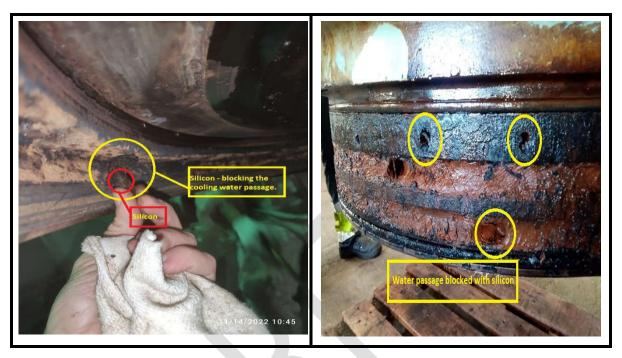
One of our fleet vessels faced issues with Jacket cooling water high temperature for one unit of Main Engine.
