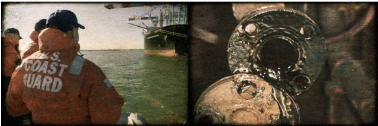
Oily bypass – checked by dismantling the overboard line connections
