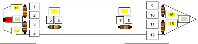
**Mooring Ropes** % Consumption & Check **End for End** Start Using Length Т % Consumption Cert. Number. Diam. **Type** Remarks Date Date **AFT STATION ( POOP DECK )** NIKA-Steel 3% GOOD & High **ROPE TAG NR. 1** 56MM 220M 12/06/19 2019/2358-6 03/06/21 tenacity 62 Polyester NIKA-Steel GOOD 3% & High 62 ROPE TAG NR. 2 56MM 220M 12/06/19 03/06/21 2019/2358-3 tenacity Polyester NIKA-Steel 3% GOOD
